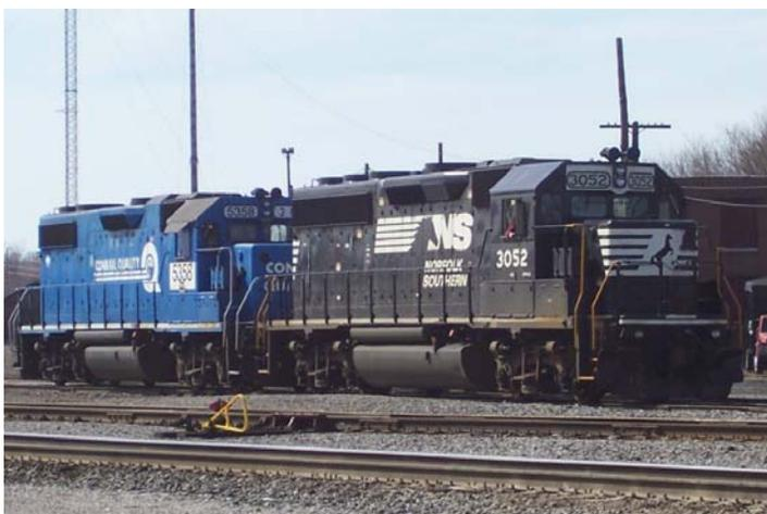
Once they had cleared the yard, the local power began switching the yard using a pair of former Conrail diesels. The blue unit is a GP38-2 and the black unit is a repainted GP40-2.
