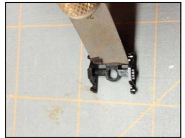
Using a chisel blade, remove draft gear just before pivot.
