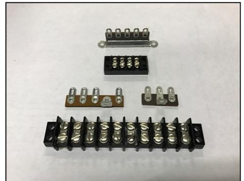
Finally there are times when your working with wires so fine they would be difficult to solder, punch down or attach to butt splice connectors. This is where screw terminals come in handy. The fine wires of block signals can easily be attached to one side of the screw terminals
