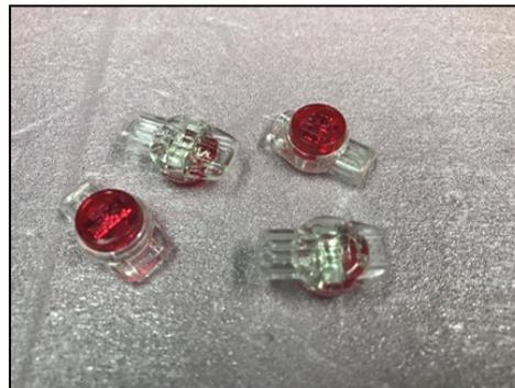
Simply insert the wires in the Butt Splice slots, compress the button on top with pliers and your connection is complete. Butt Splice connectors are available at box stores and on line. They can be purchased to accommodate two, three or four wires of various sizes from 19-26 gauge. Bulk packs of 100 are about 6 cents each. They work extremely well with typical four wire telephone cable and make a good choice for building lights, signals and accessories.
